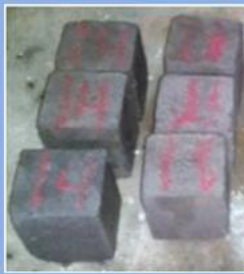
Eco Mortar using Polythene Waste
