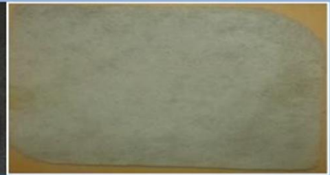
Low Cost Tiles using Cement-Sand-Slag Composite
