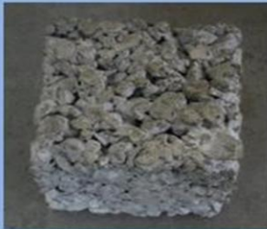
Porous Paver Block
