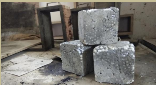
Cubes after compressive test
