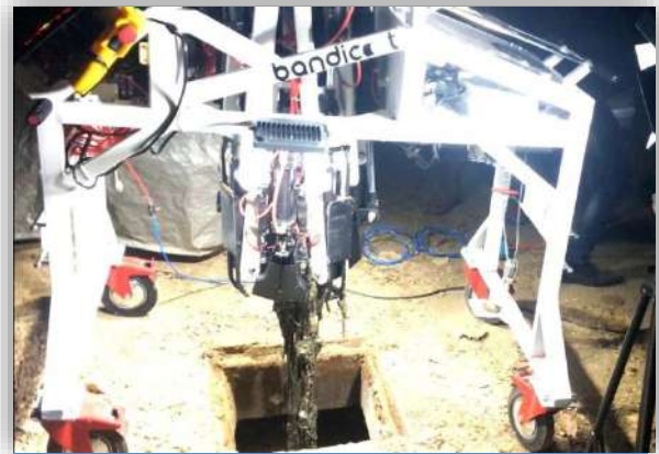
Bandicoot cleans a manhole during the trial run in Thiruvananthapuram. Photo courtesy Genrobotics
