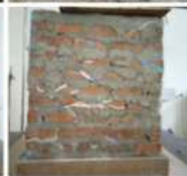
Sismic performance assessment of masonry room using uniaxial shake table at Heavy Structure lab
